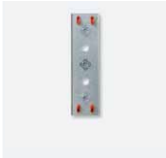
VA/GU 513-0 Vario adapter for flush-mount housing GU 513. Adapter plate to accommodate one mounting frame MR 611-3/1 and combination frame KR 611-3/1 on flush-mount housing GU 513. Hot-dip galvanized sheet steel with fastening elements for simple mounting. Dimensions (mm) W x H x D: 84 x 304 x 30
