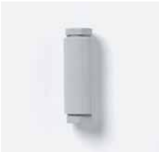
ZVM/KSA 611-0 The connecting sleeve accessory ZVM/ KSA 611-... is used as a transfer point in line with VDE regulations for the user's 230 V / 110 V mains to the BG/ SR 611-..., KSA 6... and RG/SR 611-... Mounting and accommodation in the cable channel of the standpipe or KSA. Screw union: for 5 x 2.5² according to VDE 0606 Dimensions (mm) dia. x H: 30 x 85
