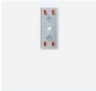
VA/GU 512-0 Vario adapter for flush-mount housing GU 512. Adapter plate to accommodate one mounting frame MR 611-2/1 and combination frame KR 611-2/1 on flush-mount housing GU 512. Hot-dip galvanized sheet steel with fastening elements for simple mounting. Dimensions (mm) W x H x D: 84 x 210 x 30
