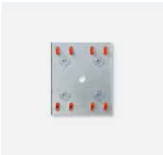
VA/GU 524-0 Vario adapter for flush-mount housing GU 524. Adapter plate to accommodate two mounting frames MR 611-2/1 and combination frames KR 611-2/2 on flush-mount housing GU 524. Hot-dip galvanized sheet steel with fastening elements for simple mounting. Dimensions (mm) W x H x D: 178 x 213 x 30
