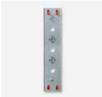
VA/GU 514-0 Vario adapter for flush-mount housing GU 514. Adapter plate to accommodate one mounting frame MR 611-4/1 and combination frame KR 611-4/1 on flush-mount housing GU 514. Hot-dip galvanized sheet steel with fastening elements for simple mounting. Dimensions (mm) W x H x D: 84 x 392 x 30
