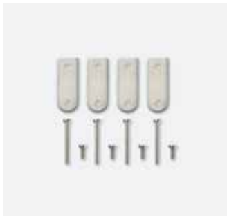
ZFB 611-0 Front panel fastening accessory for mounting a Vario DL solution in existing front panels, door side elements etc. Admissible wall thickness from 3 to 30 mm. Set contains: 4 metal brackets and 8 fastening screws for combination of VA/GU 5... in conjunction with mounting frame and relevant combination frame.
