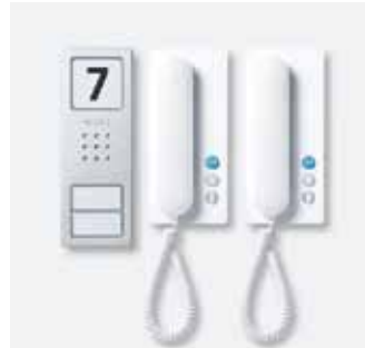
Compact Audio set: Door station for surface-mounting, with illuminated call buttons and information sign. In-house telephone with door release, light button, differentiation between door and storey calls, and call silencing.
